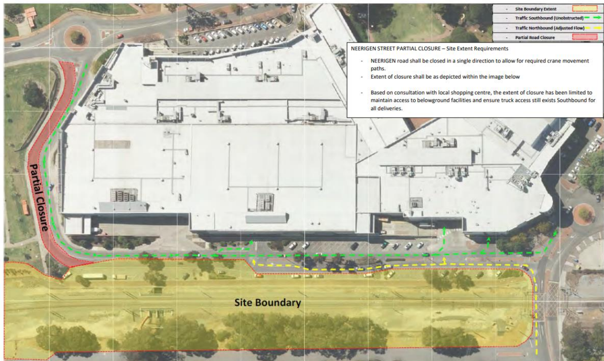
Construction Staging Concept – NEERIGEN STREET Partial Closure –
