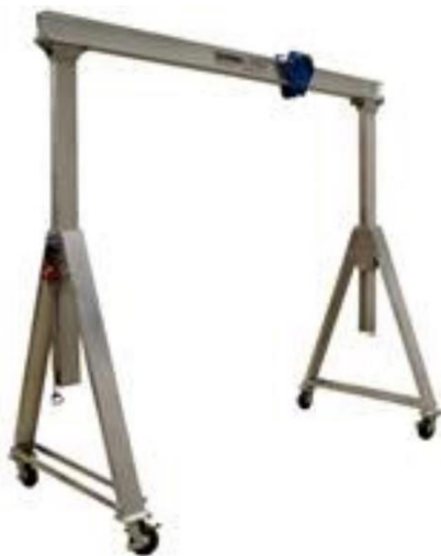
Figure 15: Example of typical lifting gantry to be used during post tensioning works on the headstock
