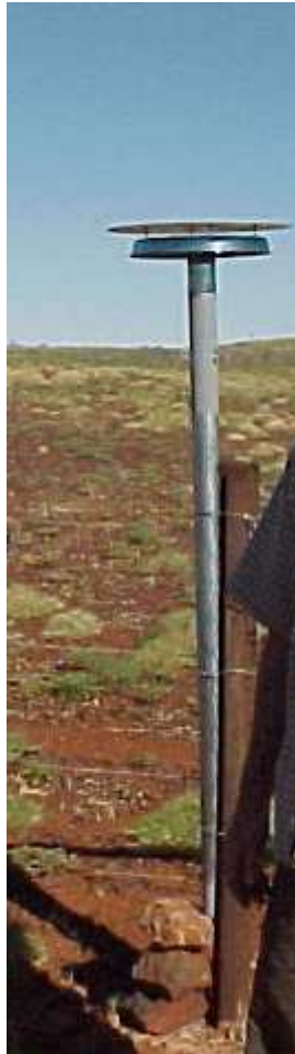
Picture 4. Installation of passive samplers under lid with aluminium radiation screen.
