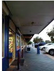
Inconsistent type, location, colour and maintenance of bollards. Exposed light fittings, poor lux readings, inconsistent lighting types and some are not in use. Signs of new and old graffiti along store face.
