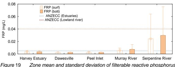
gure 19 Zone mean and standard deviation of filterable reactive phosphorus (FRP) in surface and bottom waters.
