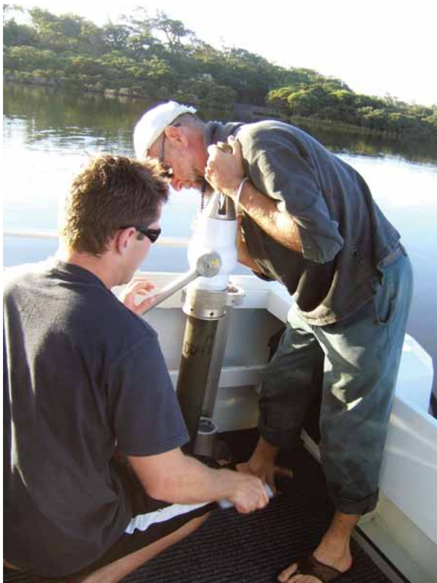
Sediment cores being collected for porosity and pore water nutrient analysis (Geoscience Australia 2008)
