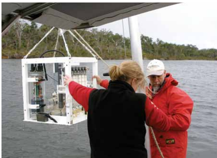
A benthic chamber being deployed in the Hardy Inlet estuary (Geoscience Australia 2008)
