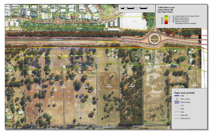
The HSA assessment acknowledged the existing limestone block noise wall and applied a wall height of 1.8m to the noise modelling. In fact, alongside Lots 242-244 the noise wall varies from 1.8m to 2.2m in height, meaning that the noise modelling can be regarded as 'conservative' and that noise mitigation achieved by a combination of the existing wall and the proposed rear setback is actually greater than shown in the modelling.
