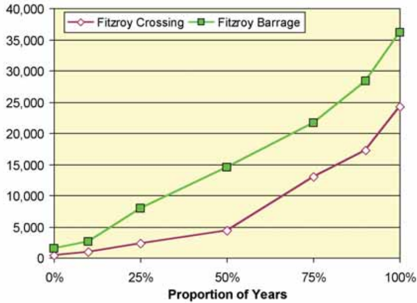
Figure 7.3 Annual Streamflow Variability at Fitzroy Crossing and Fitzroy Barrage (Liveringa) showing the proportion of years the streamflow is less than the volume shown. (e.g. 1 year in 4 the flow at Liveringa is less than 8000 GL).
