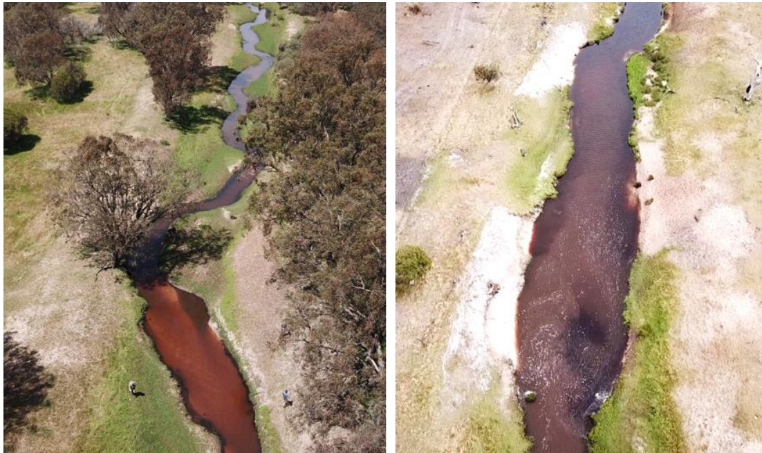
Figure 11: Visually tracking clay movement through Punrak Drain with a drone.
