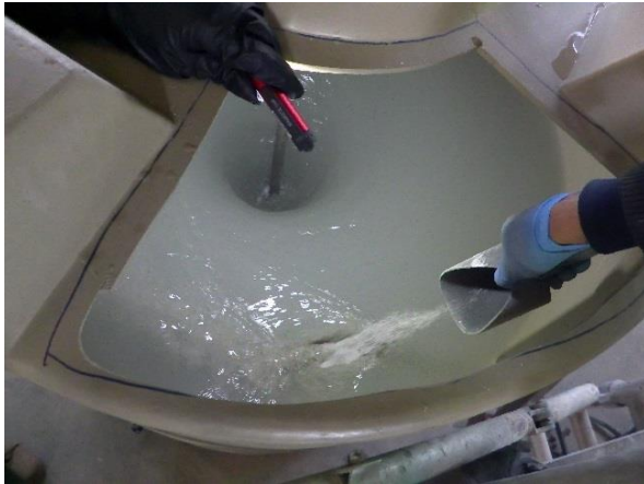
Figure 1: Production of the first larger HT-clay batch.
