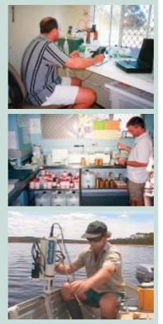
Figures 4, 5 and 6 (top to bottom): Analysing nutrient samples in a laboratory and sampling from the boat in Wilson Inlet with a Hydrolab instrument.
