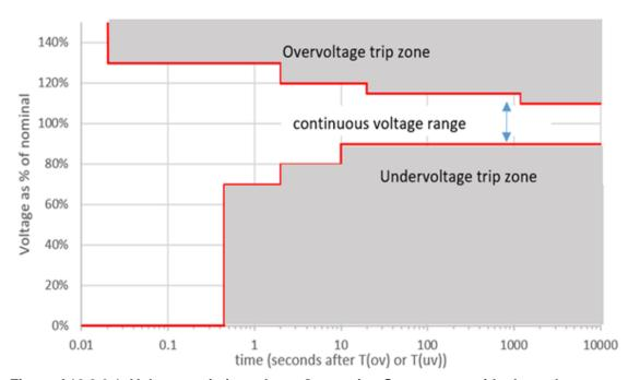
Figure A12.8.2.1: Voltage variations that a Generating System must ride through to meet the Ideal Generator Performance Standard
