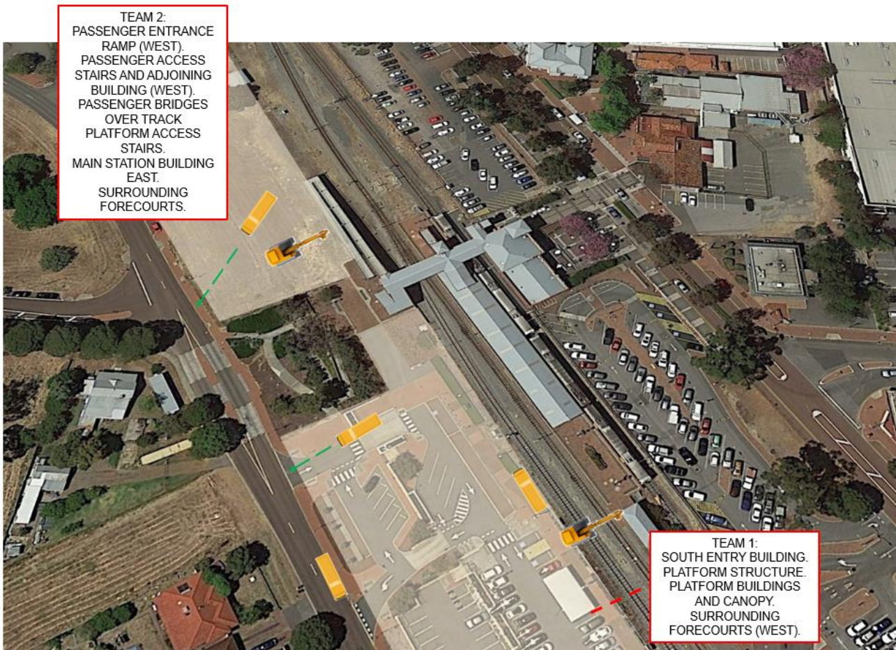
Figure 5: Armadale Station Demolition Staging
