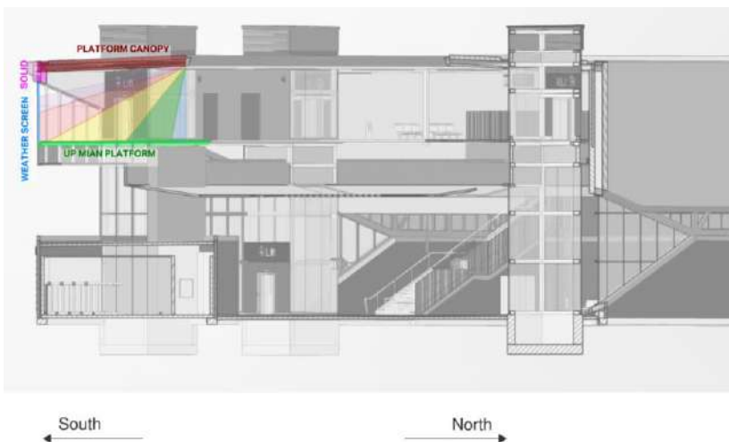
FIGURE 3-15 UP MAIN PLATFORM NORTHERN RAIN ANGLES
