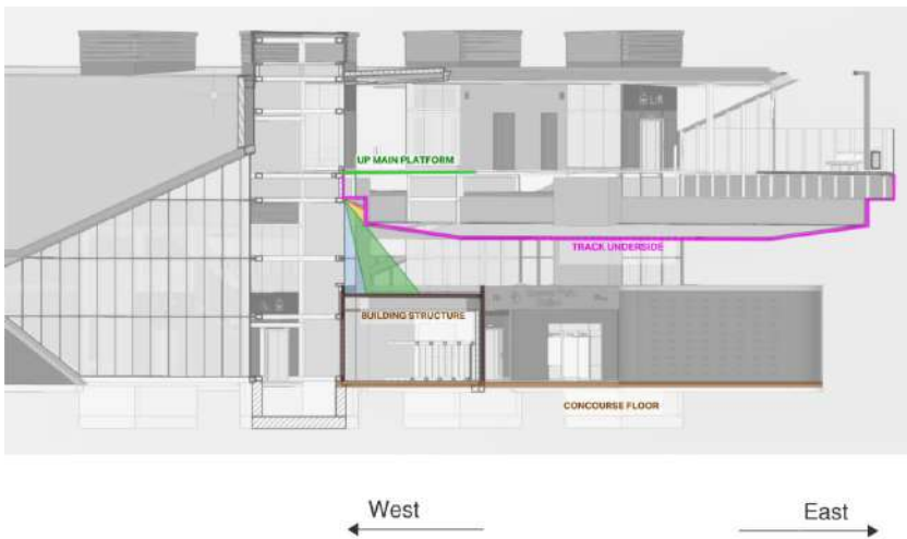
FIGURE 3-21 STATION ENTRY AND FOYER WESTERN RAIN ANGLES
