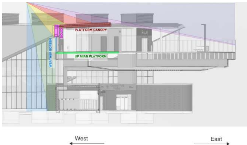
FIGURE 3-13 UP MAIN PLATFORM WESTERN RAIN ANGLES
