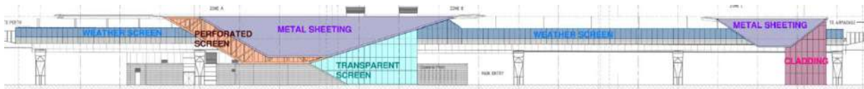
FIGURE 2-4 PROPOSED WEATHER SCREEN, PERFORATED SCREEN, METAL SHEETING AND TRANSPARENT SCREEN (WEST ELEVATION)
