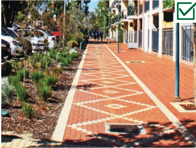
Photo 2.18 Paving pattern helps to distinguish public footpath from transition space next to the dwellings.
