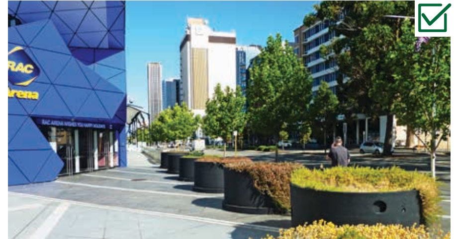
Photo 2.27 The side entrance of the Perth RAC Arena incorporates vehicle mitigation measures in the design, using large planters as bollards to provide barrier and protect the crowd when there is a performance.
