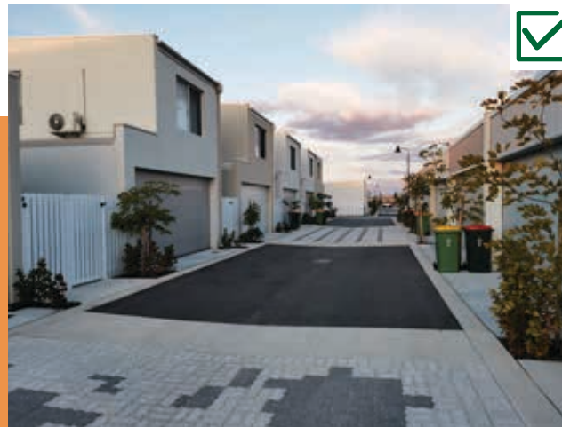
Photo 2.11 Windows above garages facilitate good surveillance to this laneway, even located just on one side.
