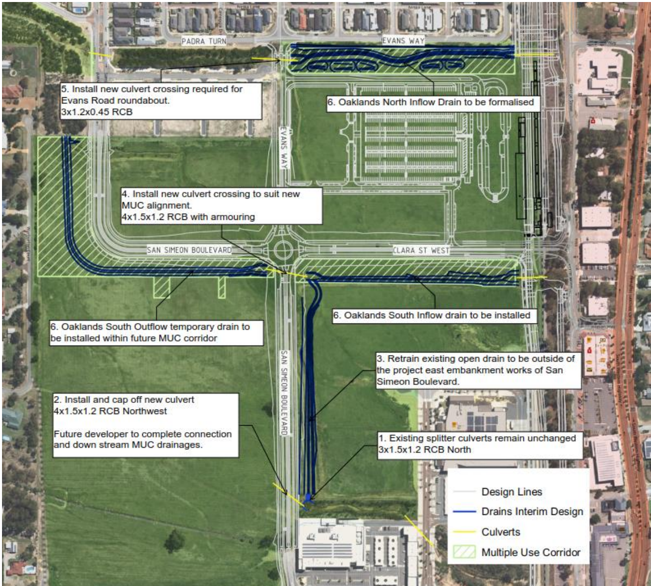
Figure 7.12. Beenyup Drain Relocation Strategy
