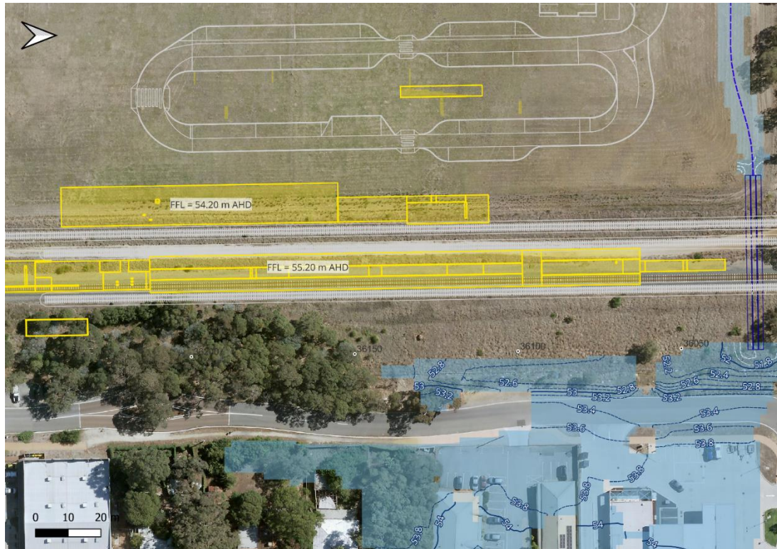
Figure 9.2: Byford Station Flood Immunity
