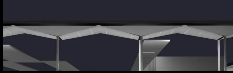
LED LINEAR PROFILES SET INTO THE PITCHED CANOPY CEILING DOWNLIGHTING PATHWAY FROM ABOVE AND BRIGHTLY LIGHTING KEY ENTRANCE AREA
