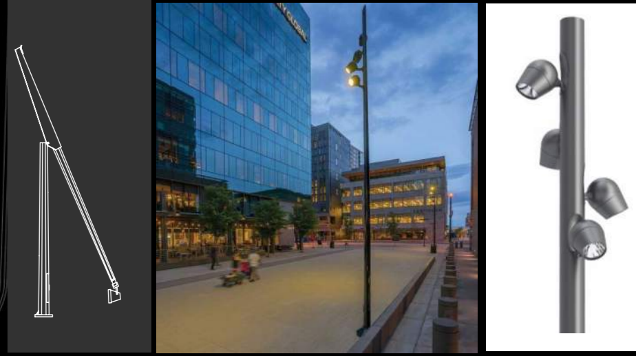
CLUSTER OF OUTDOOR SPOT LIGHTS FIXED TO 8M SEESAW TYPE POLE TO ILLUMINATE PLAZA AREAS
