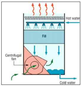
Figure 3.2 Schematic of Evaporative Cooling Tower
