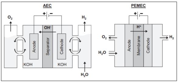
Figure 3.1 Alkaline Electrolysis Cell (AEC) and Polymer Electrolyte Membrane Electrolysis Cell (PEMEC)
