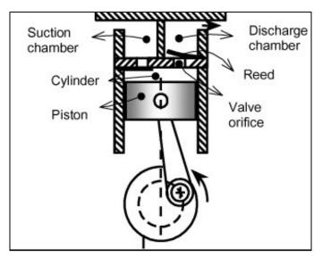
Figure 3.9 Schematic of Reciprocating Compressor
