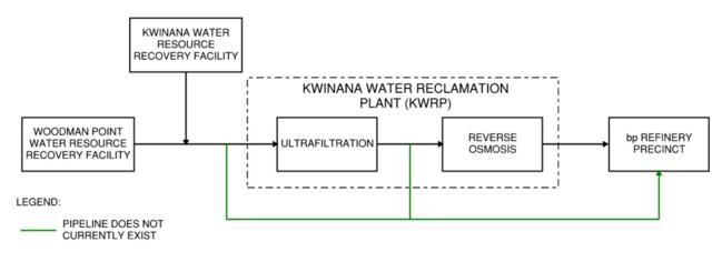
Figure 3.7 Possible Alternative Cooling Water Supply Options
