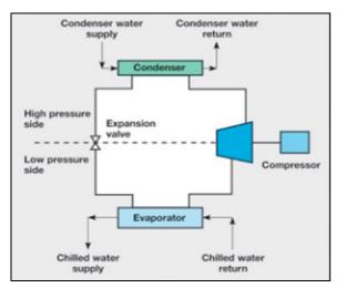
Figure 3.5 Schematic of Chiller System
