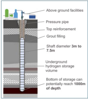
Figure 3.15 Vertical Shaft Hydrogen Storage
