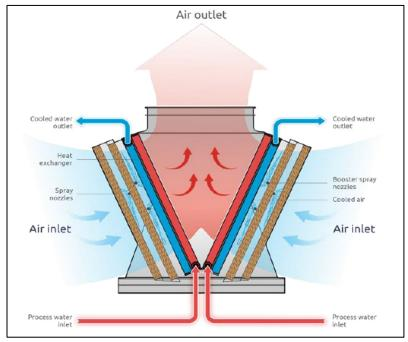
Figure 3.6 Schematic of Adiabatic Cooler
