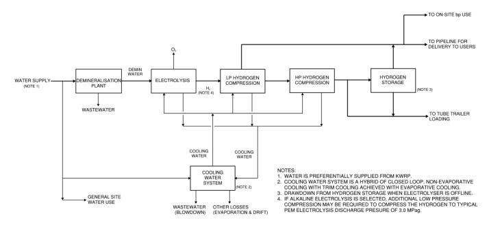
Figure 2.2 Block Flow Diagram of the Hydrogen Production Facility
