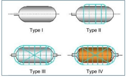
Figure 3.11 Types of Hydrogen Storage Vessels
