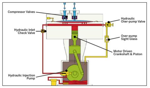
Figure 3.10 Schematic of Diaphragm Compressor
