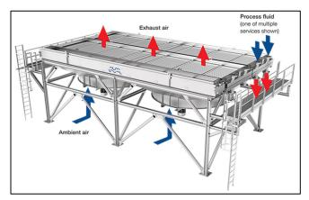
Figure 3.4 Schematic of Fin Fan Cooling
