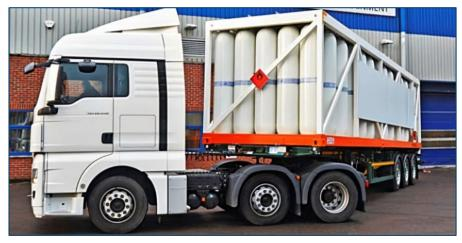
Figure 3.17 Mobile Storage Pack Loaded onto a Truck
