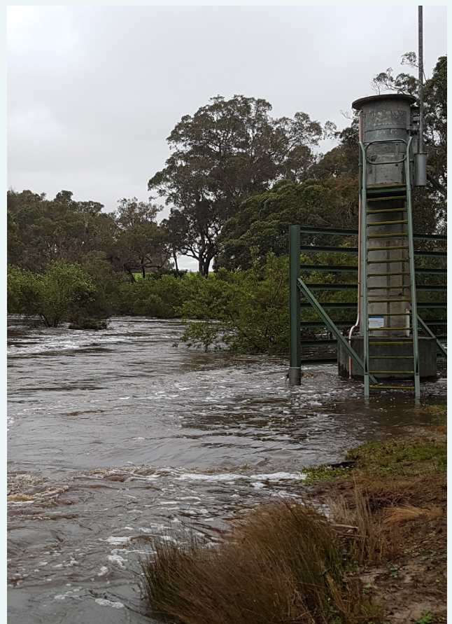
The Kalgan River gauging station during high flows, September 2017.
