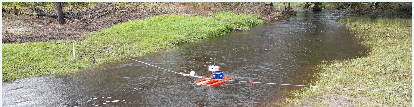
Collecting discharge measurements using a StreamPro Acoustic Doppler Current Profiler during high flows, September 2017.
