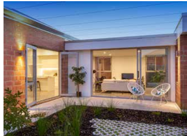
Photo G2.2b A trellis for deciduous creepers provides an alternative to a patio while permitting solar access to the primary living space (PC)
