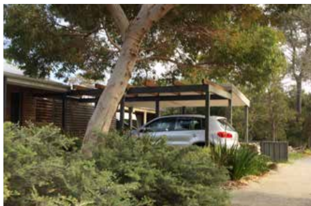
Photo G2.3c Providing a carport rather than a garage reduces the visual impact of vehicles on the street or communal area, is usually less expensive to construct, and can be located in the front setback area
