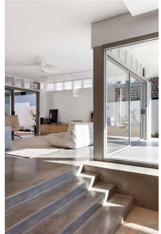
Photo G2.2c Orienting windows to the north provides effective winter passive heating to primary living spaces (PC)
