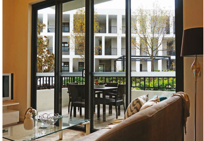
Photo 4.1b Optimising daylight access via tall windows/doors that open to a balcony/courtyard and the sky without too much recess or canopy.
