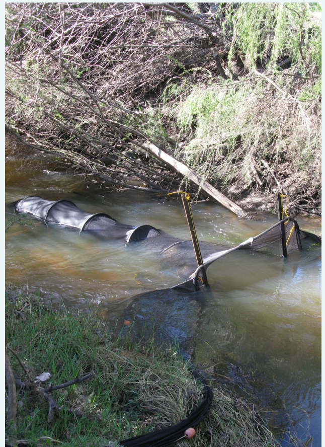
A fyke net set in the Upper Preston River to capture fish and crayfish for a river health assessment. After being recorded, they are returned to the river alive, October 2009.
