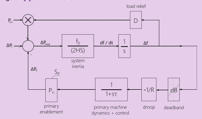
For a given set of inputs, system total kinetic energy (HS), and facility speed factor ( $\tau$ ), the required combinations of Contingency Reserve service and ROCOF Control Service are determined by numerically integrating the DFCM. From a starting frequency of 50 Hz and a contingency  $\Delta P_C$ , the DFCM is run over different levels of primary enablement ( $S_p$ ) to ensure that the Frequency Operating Standards ( $\pm$  any Margin for Operation) are exactly met.
