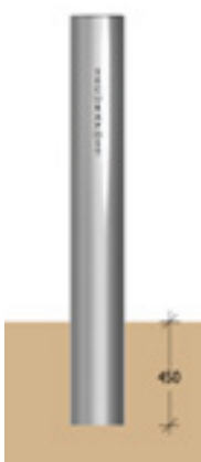
Bollard Type 1 – Fixed
