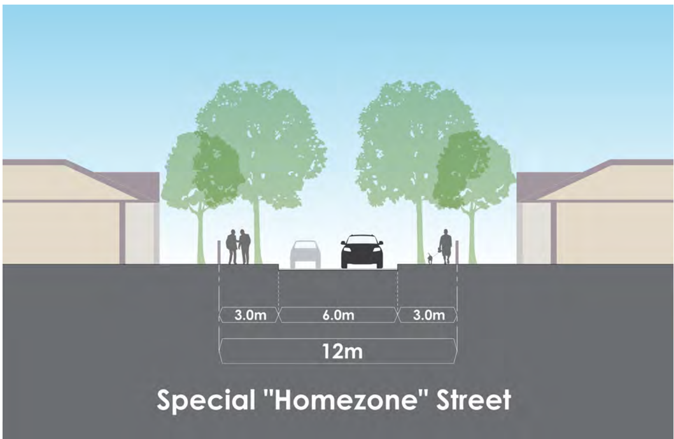
Figure 11 Special "Homezone" Street Indicative Cross-Section
