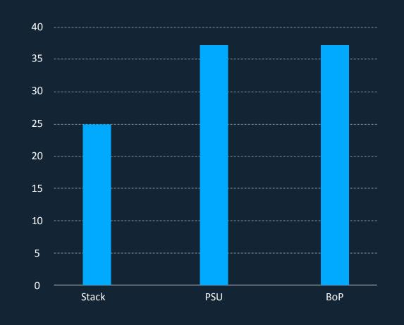
(Figure 21) PEM electrolyser major cost drivers as a percentage of unit cost
