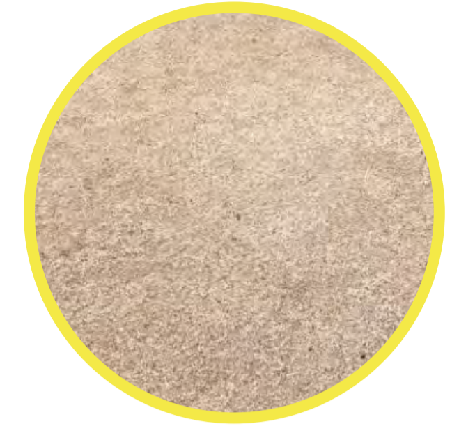
INFORMAL PATHWAY COMPACTED LIMESTONE 5% CONCRETE MIX
