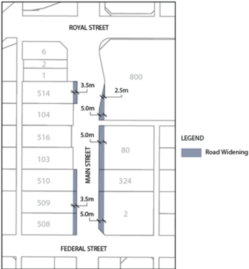
Figure 6.18.4 – Road Widening Plan
