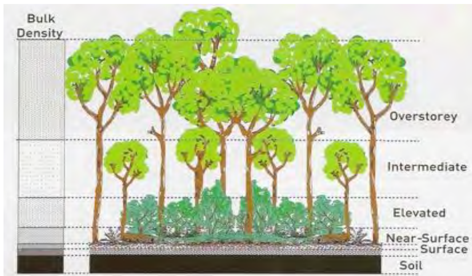
Plate 2: The five fuel layers in a forest environment that could be associated with fire behaviour (Gould et al. 2007)
