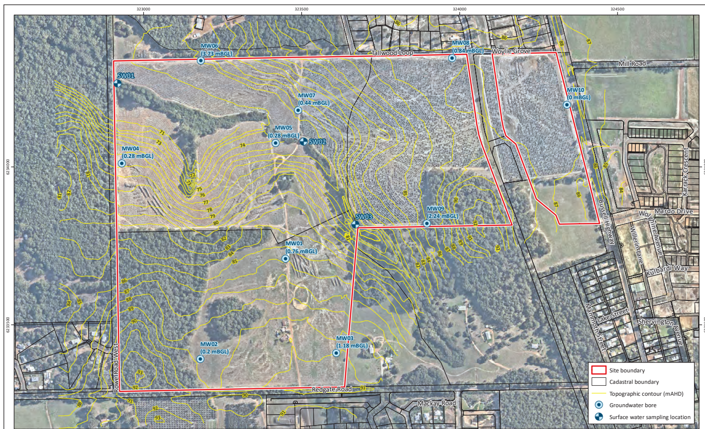
Figure 2: Topographic Contours and Groundwater Levels
