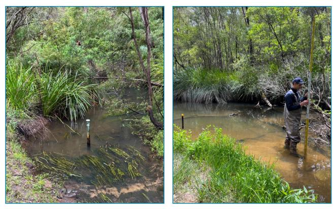
Figure 9 Surveying ecological features and installation of water level loggers at two environmental flow study sites in the Warren River catchment.
