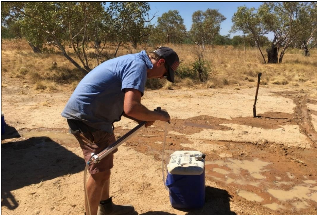
Figure 25 Groundwater sampling for noble gases, using the copper tube method
