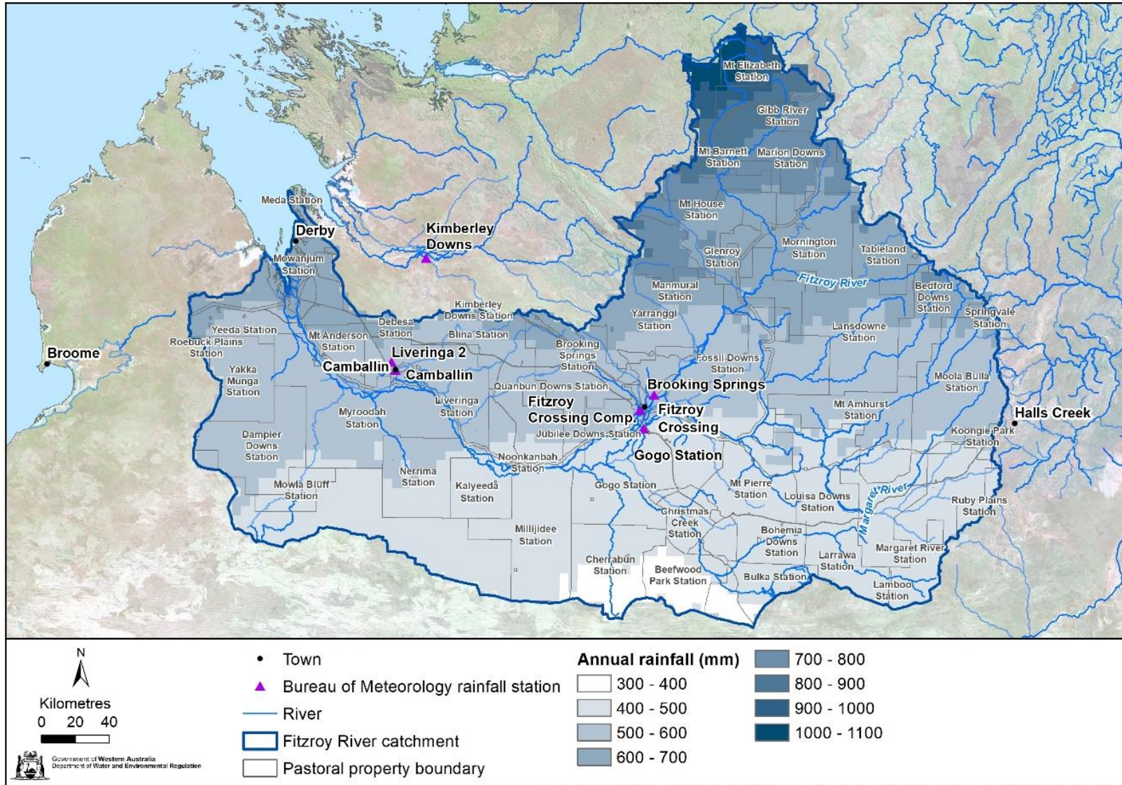
Figure 11 Bureau of Meteorology rainfall monitoring sites and rainfall gradient across the catchment
