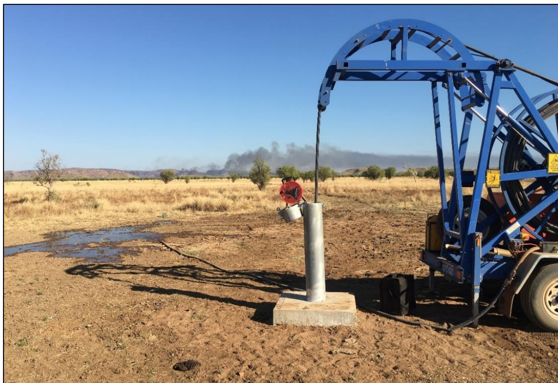
Figure 23 Groundwater sampling using pump trailer at LF02
