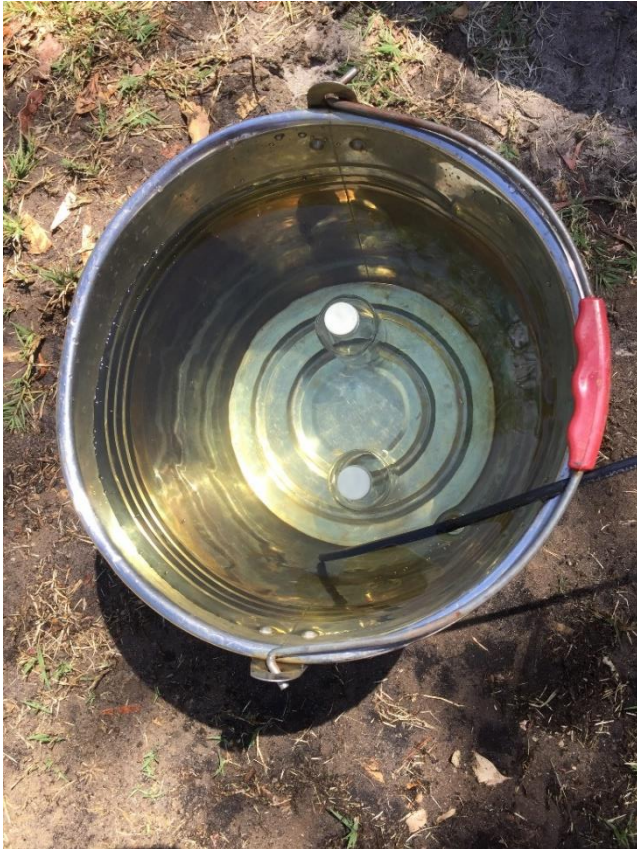
Figure 24 Groundwater sampling for CFCs
