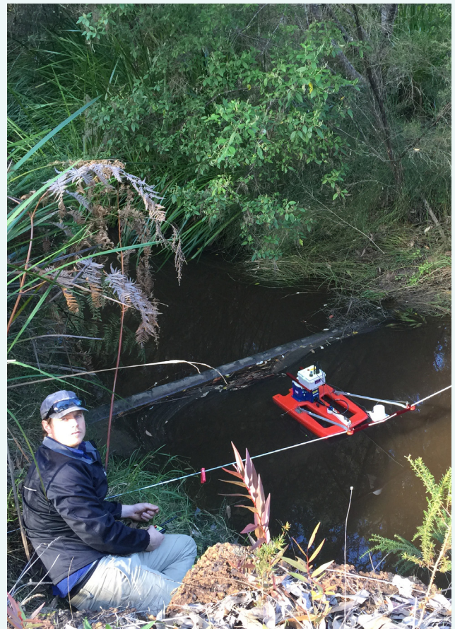
Collecting flow measurements using a StreamPro Acoustic Doppler Current Profiler, July 2016.
