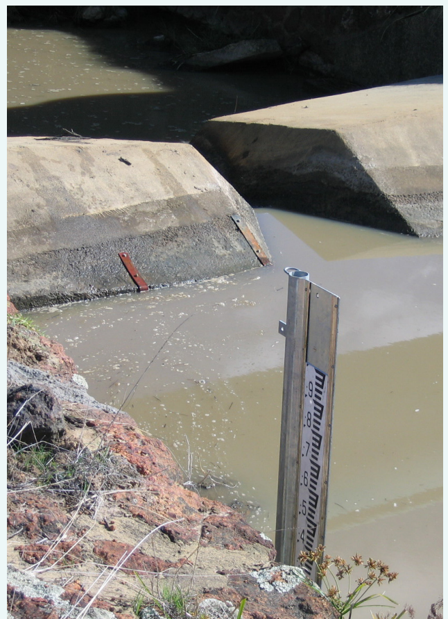
The staff gauge and weir at the Samson North Drain sampling site, May 2006.
