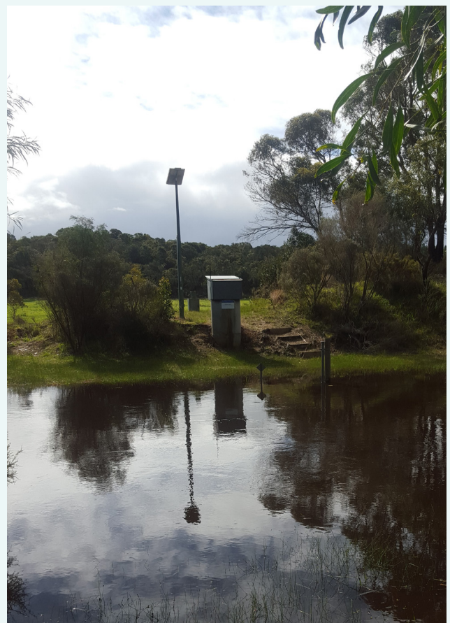
The gauging station at the Sleeman River sampling site during very high flows, August 2017.
