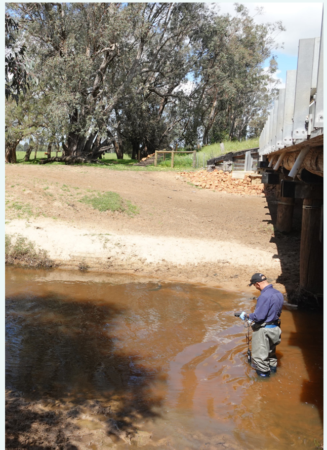
Using an in-situ probe to measure pH and salinity at the South Dandalup River sampling site, September 2018.
