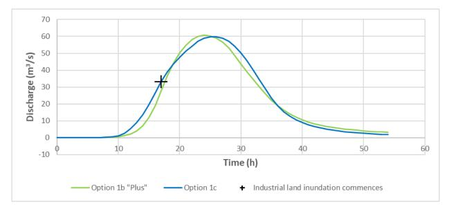
Figure 34 Cell 6 discharge for Scenario 1 Option B Plus and Option C
