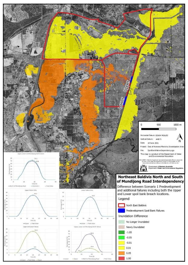
Figure 41 Scenario 2 spoil bank failure sensitivity 1% AEP flood
