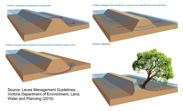
Figure 6 Sample of failure mechanisms considered by desktop assessment
