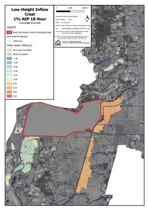
Figure 38 Scenario 2 potential 1% AEP flood low-height inflow crest at 10.3m AHD
