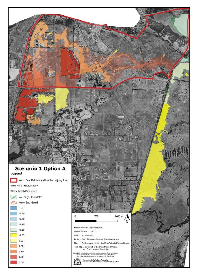
Figure 36 Pre-development 5% AEP flood spoil bank failure sensitivity
