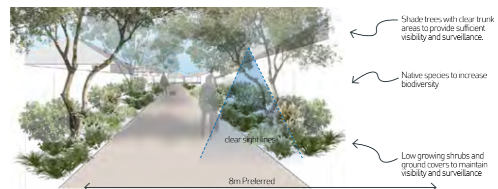
P2 - Figure 27: Typical section Pedestrian Access Ways
