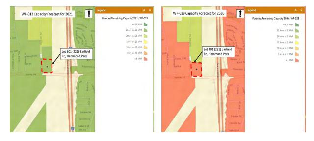
Figure 17 Western Power Remaining Capacity Forecast
