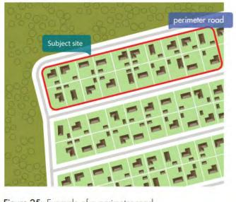
Figure 25: Example of a perimeter road
