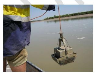
**Plate 1.** Collecting sediment samples at EST03 with an Eckman-Birge grab sampler.
