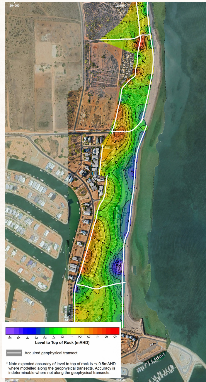
Example contour map showing estimation of bedrock elevation
