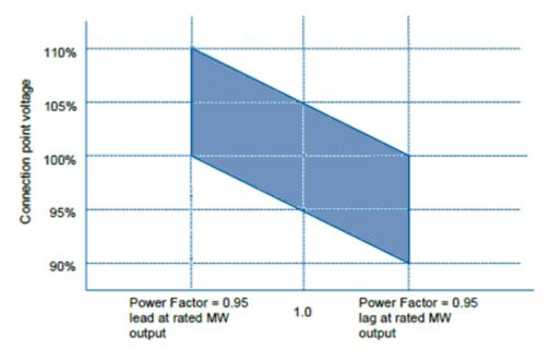
Figure A12.3.3.2: Relaxation of Reactive Power requirement with Connection Point voltage
