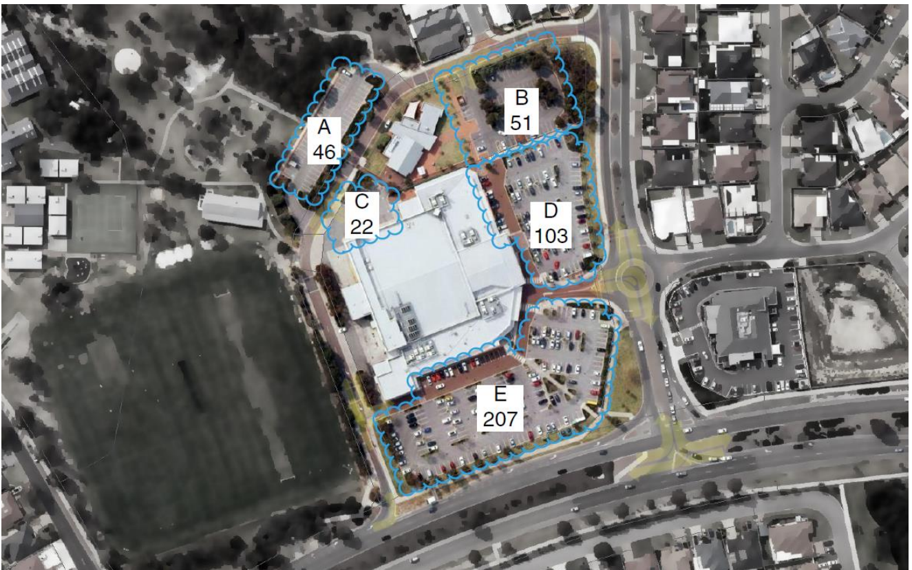
Figure 9 Car parking cells and yields. Cells C, D and E are located on the subject site.
