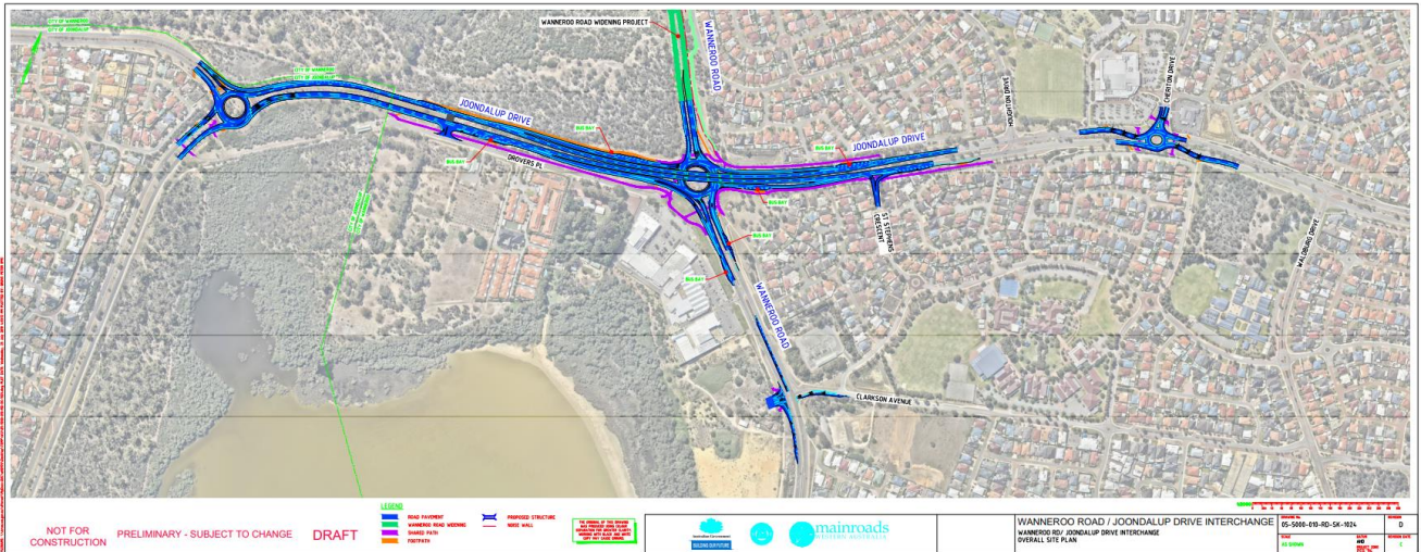
Figure 10 The roundabout will improve traffic flow of vehicles existing Cheriton Drive onto Joondalup Drive. Wanneroo Road / Joondalup Drive Interchange Overall site plan Extract July 2018
