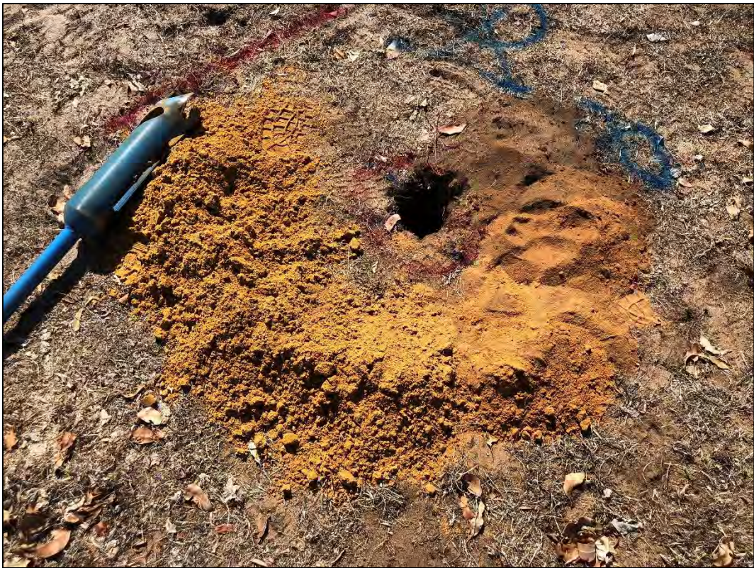
Figure 2: Borehole arisings from HA7
