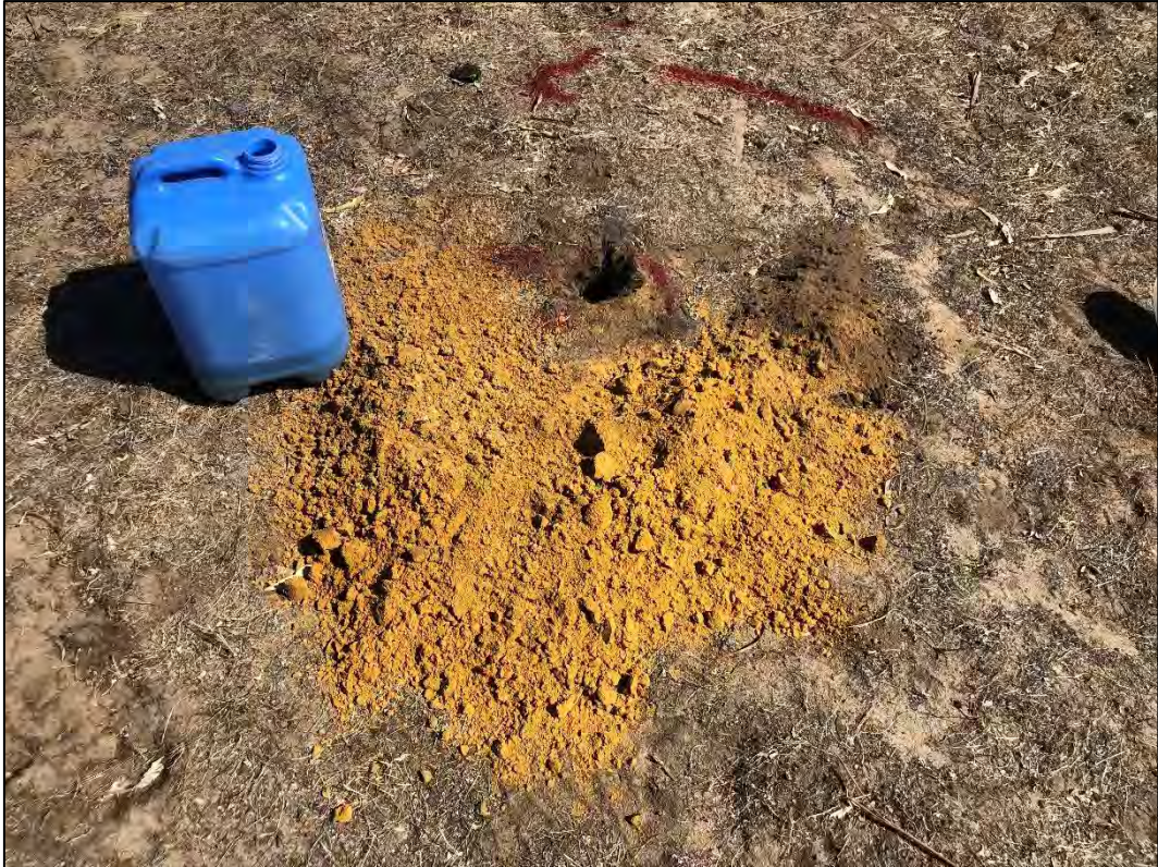
Figure 3: Borehole Arising from HA6
