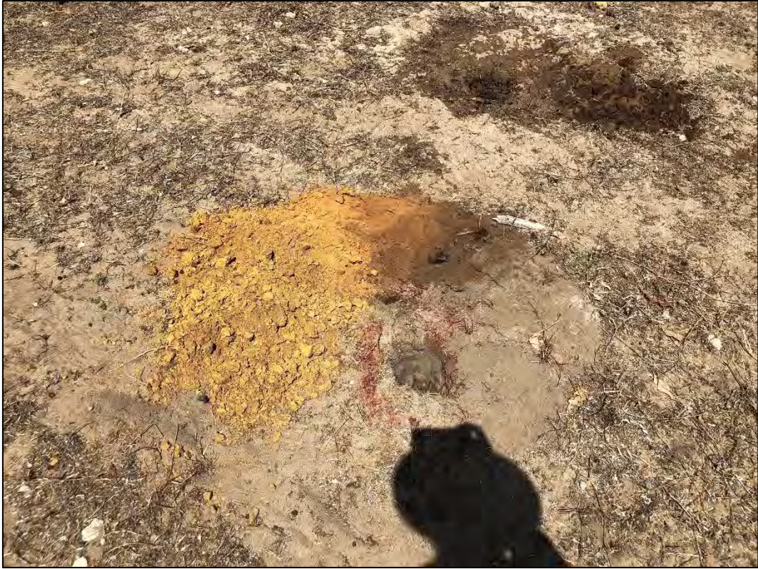
Figure 1: Borehole Arising from HA1
