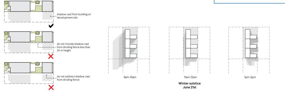
Figure G3.9a Dividing fences excluded from overshadowing calculations
