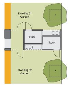
Figure G2.6a Outbuilding as a boundary wall
