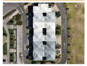
Photo G2.10b Consolidated vehicle access points reduce crossovers to the street and allow for street parking
