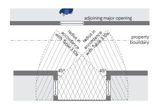
Figure G3.10a Window placement to avoid direct overlooking
