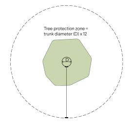
Figure G1.2a Establishing a tree protection zone
