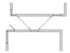
**Figure 59** Increased fence heights or offsetting of windows are measures that may prevent overlooking
