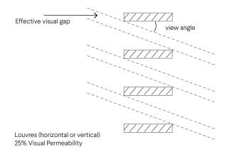
to achieve acceptable screening will depend on the view angle and width of the louvre blades, suitably interrupting the line of sight (refer **Figure G3.10d**).
