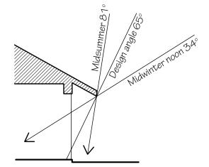
Figure 70 Calculated eaves overhang on north side, Perth
