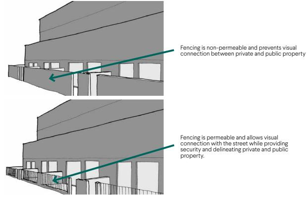
Figure 35 Fencing should not impede visual surveillance of the street by either being too high and/or non-permeable
