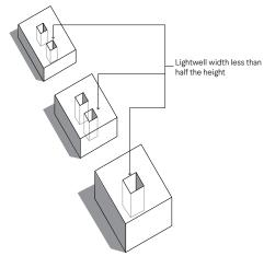
Figure G2.2b Lightwell width to height ratio
