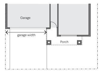
**Figure G3.6a** Piers and porches forward of garages excluded from garage width calculations.
