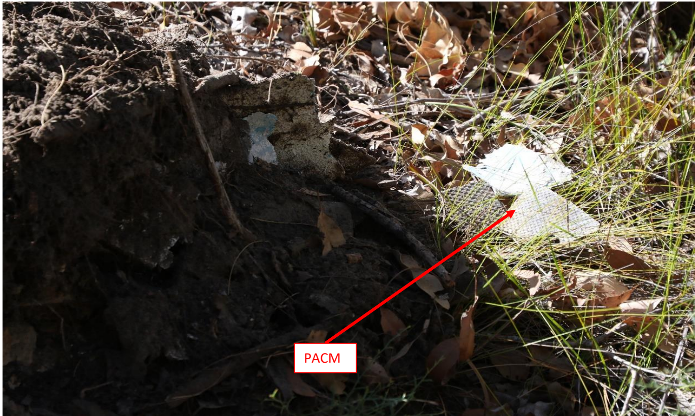
Photograph 12: Feature 6 - potentially asbestos containing material in spoil
