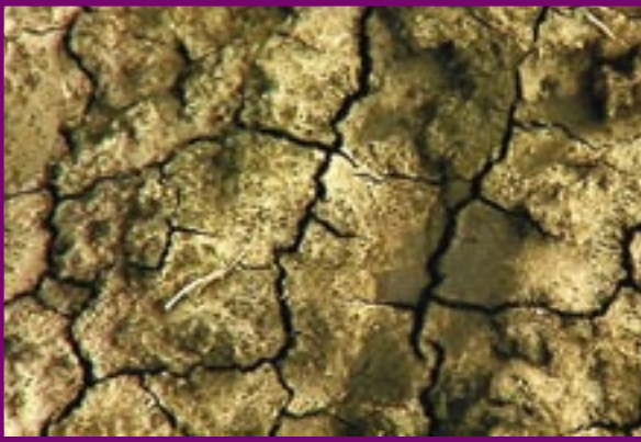
Fig 23. Desiccation cracks in clay (Reference 24)
