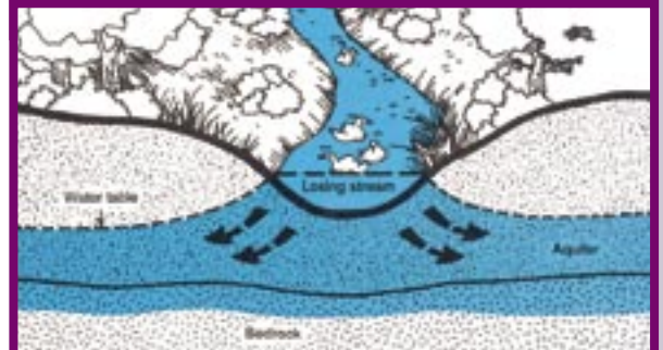
Fig 13. Groundwater. Gaining streams and losing streams (Reference 8)
