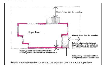
7.1.13 Balconies or decks at an upper level may be located within 4.5m of the boundary to an adjacent lot where the wall is equal to greater than, 75 degrees to the boundary, provided that the balcony does not project beyond the face of the wall.
