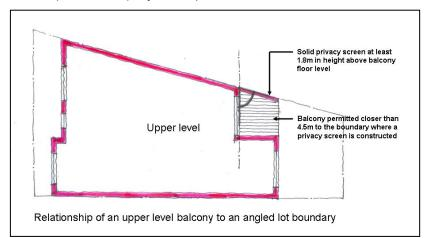
7.1.14 Where a balcony or deck at an upper level is located within 4.5m of a boundary with another lot, the balcony shall incorporate a permanent solid vertical screen to a height of 1.8m above the finished floor level on the side of the balcony facing the adjacent property.
