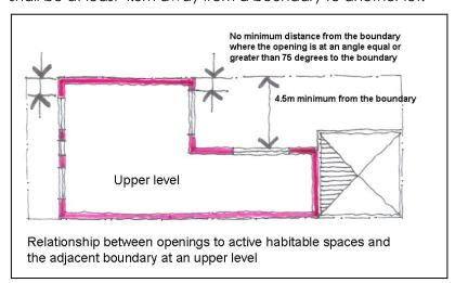
7.1.10 Major openings at all upper levels including the split levels may be located within 4.5m provided the sill level of the major opening is at least 1650mm above its finished floor level.
