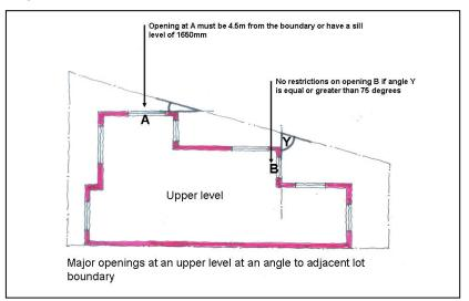
7.1.12 Balconies or decks at an upper level shall be located at least 4.5m from the boundary, except as described in clauses 7.1.13 and 7.1.14 below.
