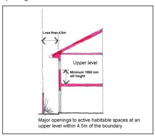
7.1.11 No minimum distance from the boundary where the major opening is situated in a wall at an angle greater than 75 degrees from the boundary.
