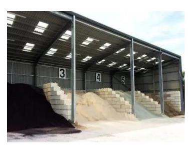
The height of aggregate or sand must not exceed the height of the storage bin or bay, including any windshields fitted.
