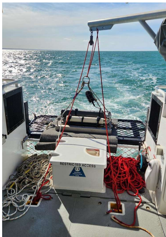
Figure 5. (Left) Baseplate with Autonomous Multichannel Acoustic Recorder (AMAR), external battery, and hydrophone on the aft platform of the Optimus , with ground line (white) and lowering line (red) prepared for deployment in the Exmouth Gulf. (Right) AMAR G4 in acetal housing.
