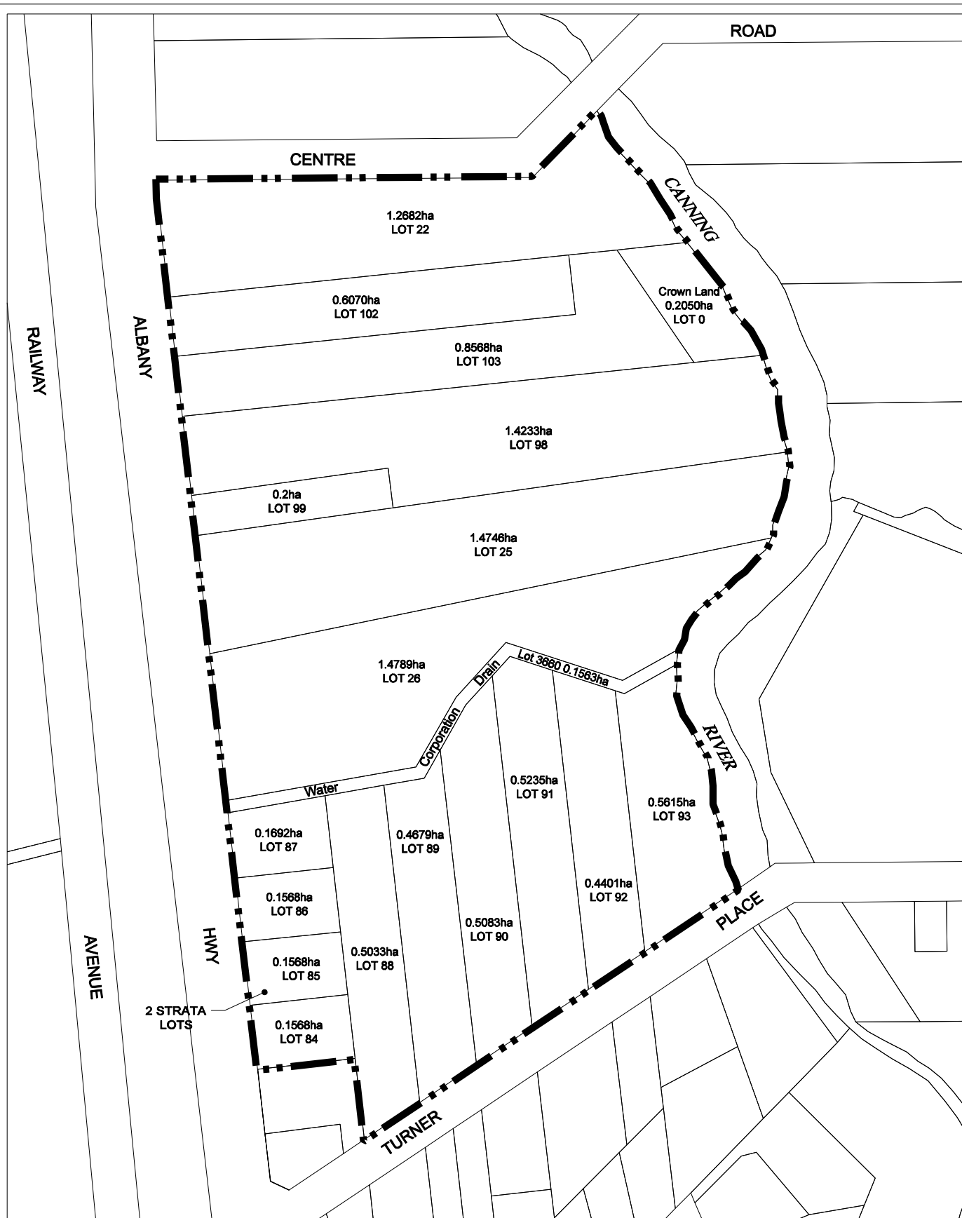
LOT CONFIGURATION & AREAS - FIGURE 2 CENTRE ROAD CANNING RIVER (WEST) URBAN STRUCTURE PLAN
