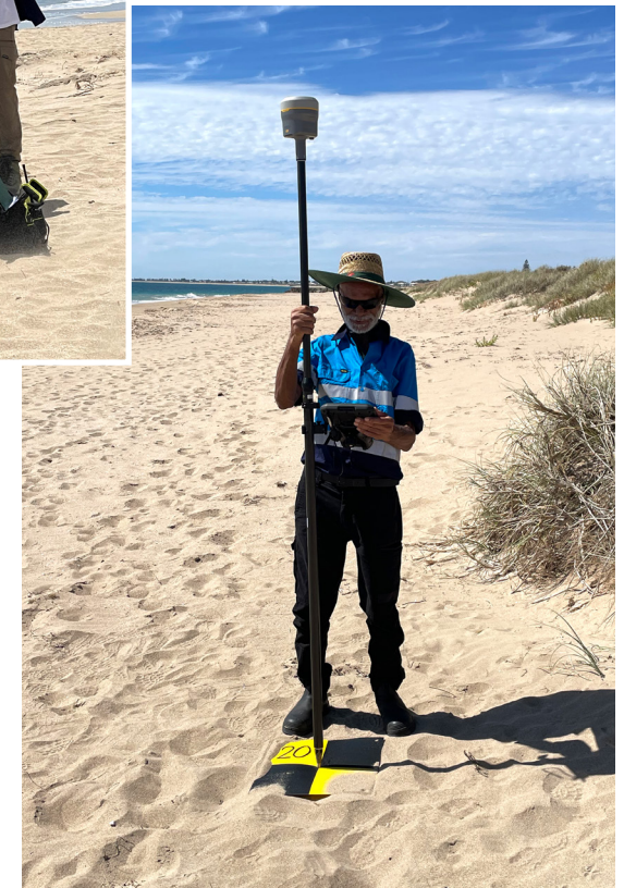
Drone team member conducting GPS survey of beach control (image sourced from DoT)
