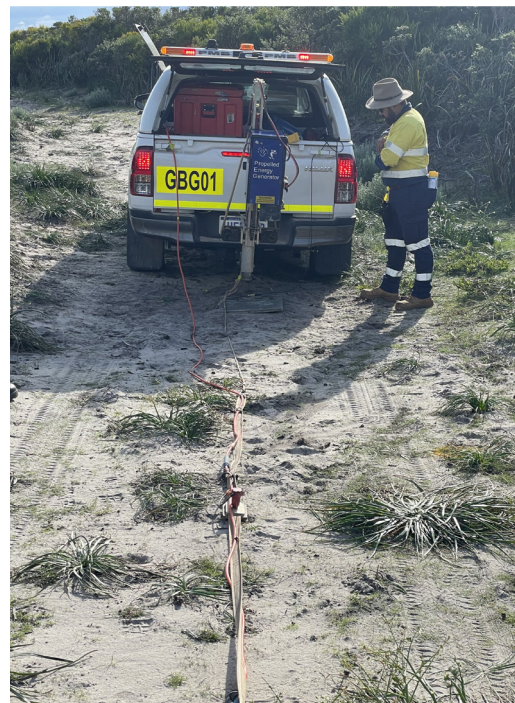
Geotechnical survey underway with Geophones laid out and used to record sound waves reflecting on underground rock layers (images sourced from DoT)
