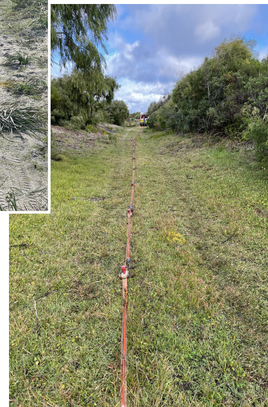
Geotechnical survey underway with Geophones laid out and used to record sound waves reflecting on underground rock layers (images sourced from DoT)
